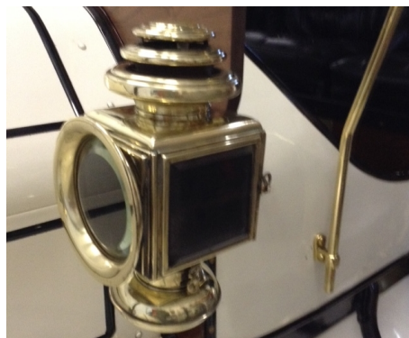
Photo #4 Chadwick Bros cowl lamp as used on Canadian built E-M-Fs
