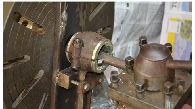
Photo 3: Jig for machining rod bearings on the lathe
