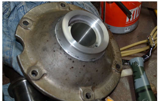
Trans-axle part machining completed.
