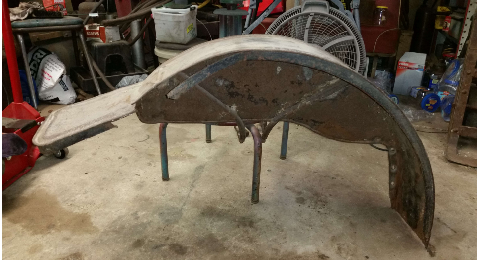
Right rear fender of the editor's 1912 E-M-F Demi Tonneau before much restoration work started. Note that the back of the fender should be parallel to the ground.
