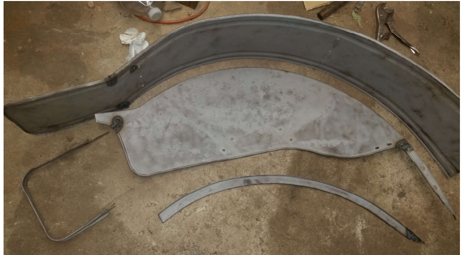
Right rear fender disassembled and its parts laid out on the garage floor. Notice I had started reshaping the fender and welding up cracks.
