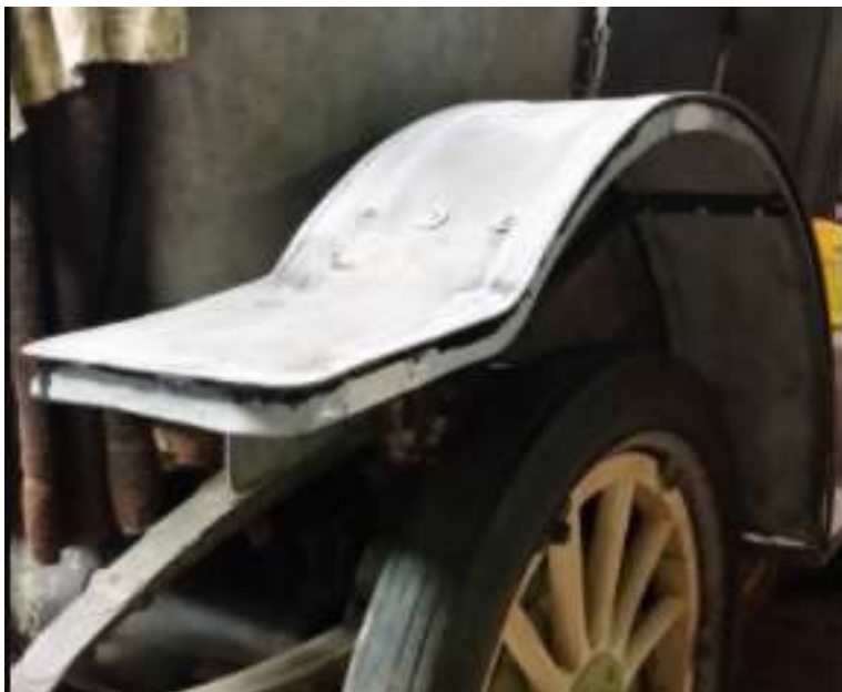
Right rear fender reassembled checking for fit on the car
